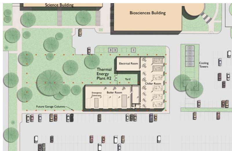
Thermal Energy Plant No. 2 Site Plan
