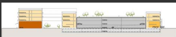
Parking structure with building liners
